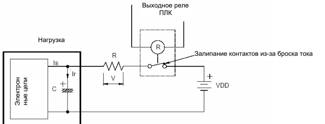
$$R \geq \frac{V_{DD}}{I_{r\ max}}$$
