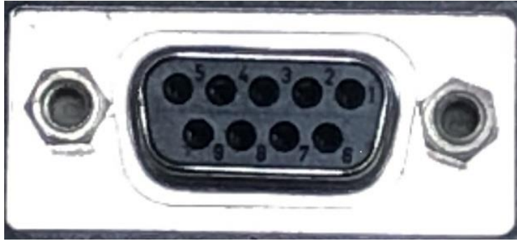
Figure 8 Siemens S7-300 communication interface
